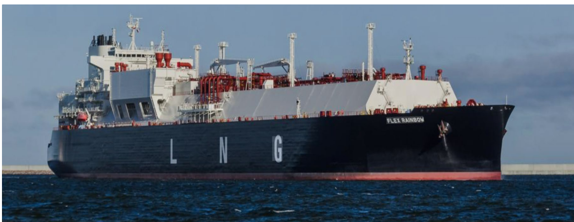
The Flex Rainbow LNG carrier, with a capacity of 174,000 m 3 . This tanker has been fitted with GTT's Mark III Flex membrane system. Image: © GTT
